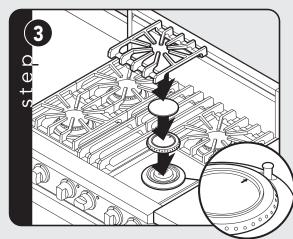
Burner caps are packed in styrofoam top pack with the grates.
